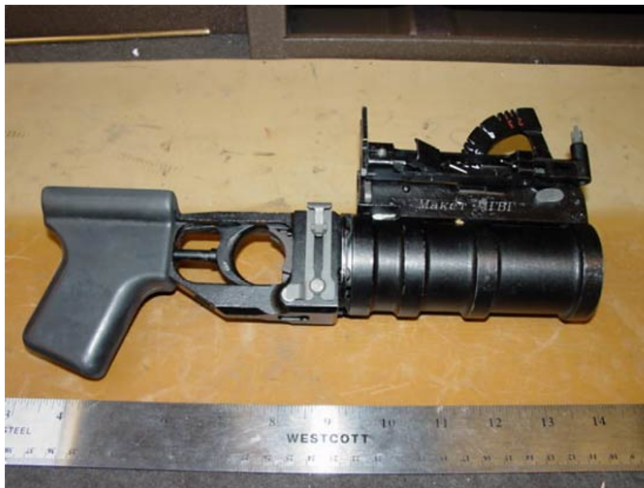
Russian GP-30 40mm grenade launcher
