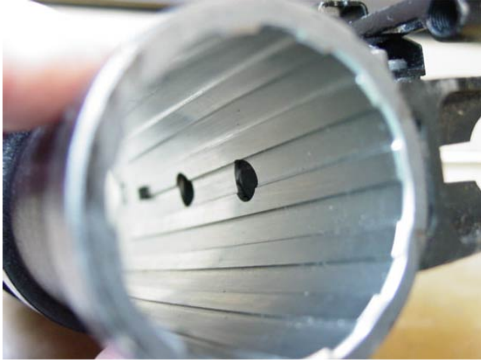
Barrel alteration (interior view)
