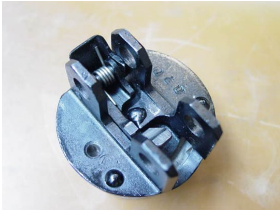
Breech (rear view, showing spot welded firing pin)
